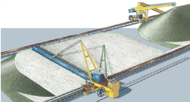
Figure 3.2.11. Strata storage method. Lateral scraper.
