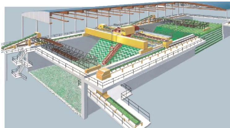
Figure 3.2.17. Windrow method with pit preblending system.
