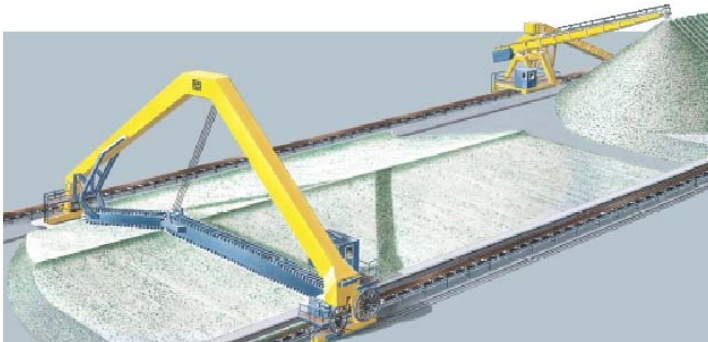
Figure 3.2.10. Strata storage method. Full portal scraper.
