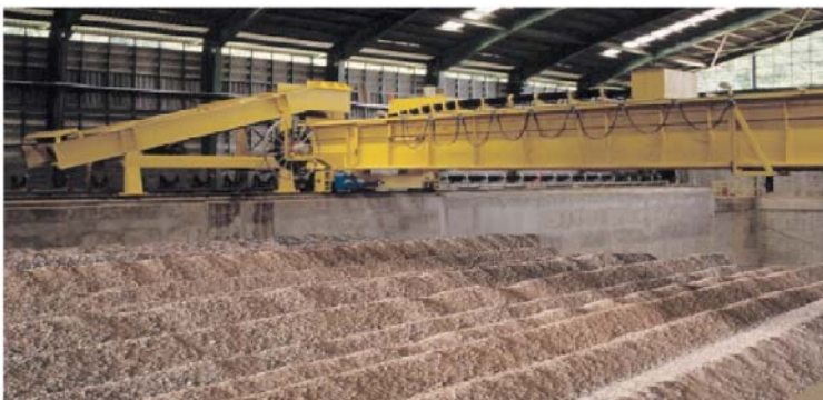
Figure 3.2.16. Chevron method with circular preblending system for continuous stacking.
