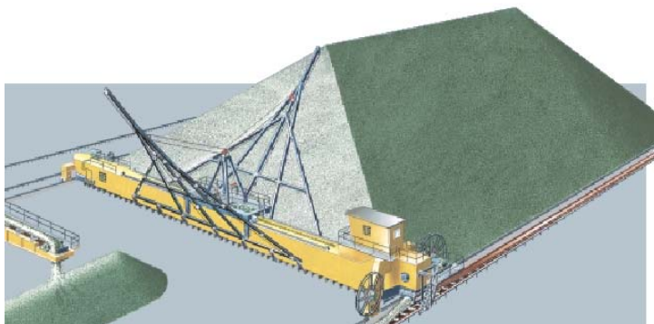
Figure 3.2.15. Chevron method with longitudinal preblending system.
